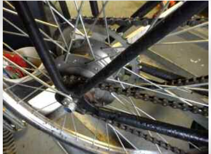
Well you can't see much but the freewheel thread on the hub is stripped, thus ruining the hub
