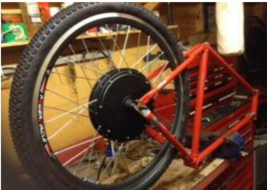
**Dry fitting of the Electric motor wheel prior to going to the paint shop.**
