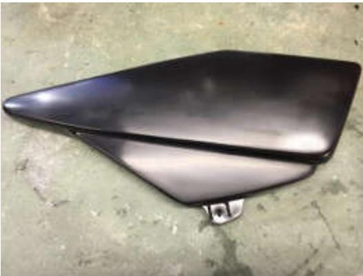
This is our workpiece today- freshly plastic welded and painted in basecoat black. Even though the paint is fresh a clean workpiece and environment is essential to getting a satisfactory result, lumps of dust under decals just don't look nice! To make matters worse peeling off the backing paper will generate a static charge,
