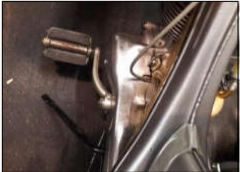
**Quickly - Left Hand pedal and crank**
