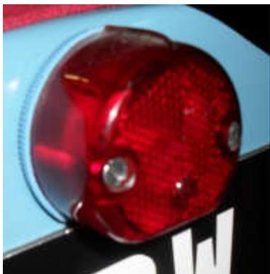
Finally I used small diameter bolts through the lens body long enough to also bolt the whole assembly to the number plate with these same bolts.
