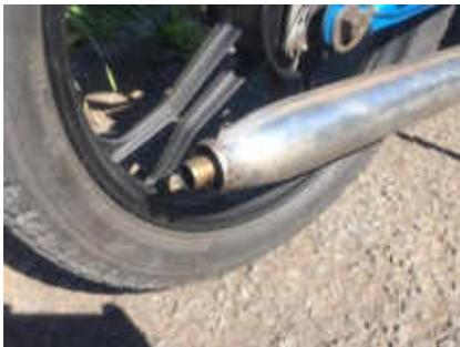
The exhaust port exit angle of the Puch is different from the Tomos, so I had to fabricate a suitable front pipe to mate up with the standard Tomos item.
