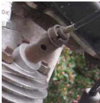
Meantime.... the technique with these engines is to set the friction drive on your tyre, peddle away with the motor in decompression mode then slowly move the throttle lever forward to close the decompression valve and open the throttle – yes one lever does it all. By great good fortune, Mark Daniels, the same genius who helped me with the Benelli engine has supplied me with that cunning period control lever. My problem whilst waiting for parts has been how to fabricate the Bowden cable
