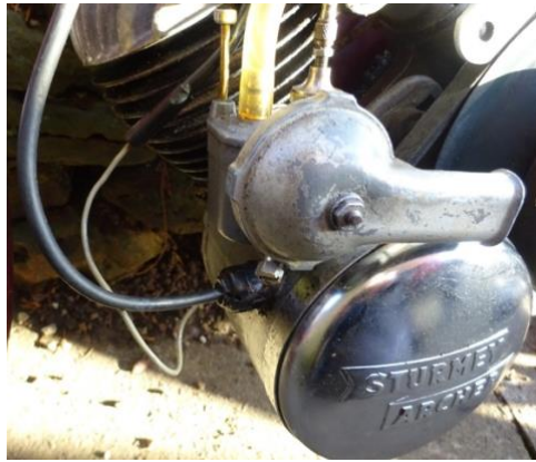
The Amal carburettor as fitted to the Raleigh RM2
